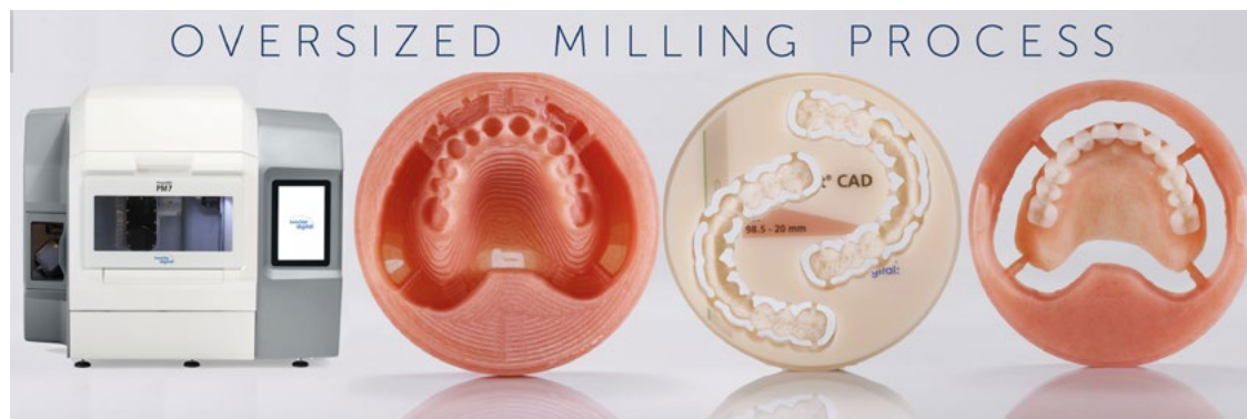
Figure 23. The oversized milling process has changed digital denture manufacturing process efficiencies, as well as the accuracy, predictability and overall strength of the restorations. The Ivoclar Digital Denture System has a milling process that provides all of these aspects, the unique "Oversized Milling Process," which eliminates the need for manual removal of excess bonding material. The tooth arch and denture base are milled to approximately 80%, with the base sockets and tooth necks milled to precision. The arches are then bonded together, and the prosthesis is put back in the mill for a final milling.
