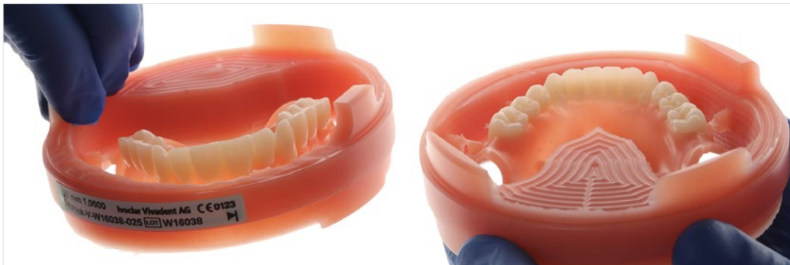
Figure 29. Results of the milling process directly after milling in the PM7. Note the incisal translucency achieved with the Vivodent CAD Multi.
